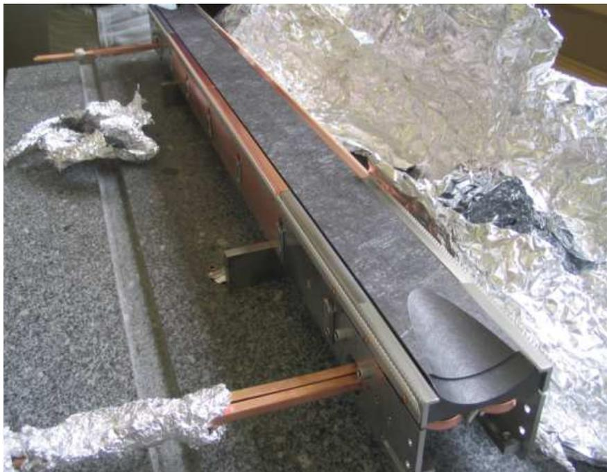
Figure 2.11: Carbon collimator jaw used in LHC collimators.
