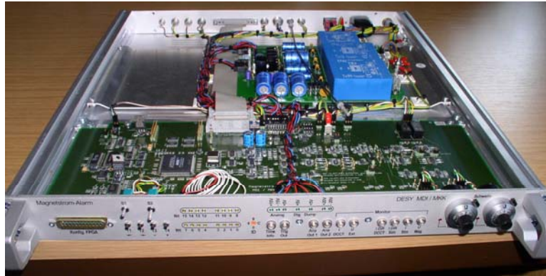
Figure 1: DESY version of the Fast Magnet Current Change Monitor (before CERN adaptation; in the back the power supply and in the front part the analogue electronics and the FPGA)
